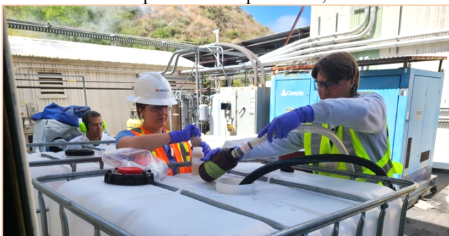
Figure 2. Collection of treated effluent for PFAS analysis.
